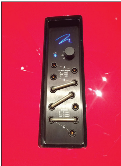
Detail view of the Neolith's jumpers—located on the rear of the speaker. Low bass was set to zero and distance was set to 4 meters.
